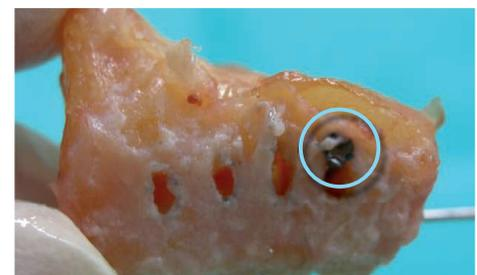
Figure 5: Distal fragment post test after removal of plate 3 showing 'long holes' and broken screw (blue circle)
