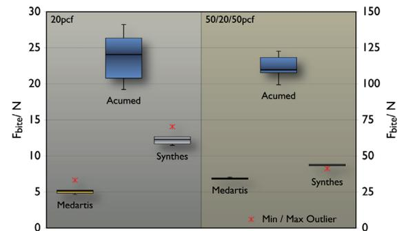
Figure 2: Bite force of different screws in two substrates (Sawbones 20 pcf and 50/20/50 pcf); lower values are better
