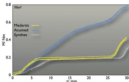
Figure 3: Insertion behaviour of different screws in Sawbones 20 pcf substrate; lower values are better
