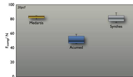
Figure 4: Compression of different screws in sawbones 20 pcf substrate; higher values are better
