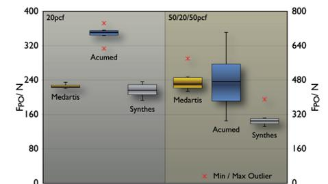
Figure 5: Pull-out force of different screws in two substrates (Sawbones 20 pcf and 50/20/50 pcf); higher values are better
